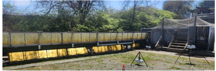
Image 4. The USGS Conte lab, facility to test fish swimming performance of migrating fishes (Ted Castro-Santos lead). The long flume (left) can adjust rates of flow, velocities and fish leave the tanks on right under their own volition, when test trials are run.
